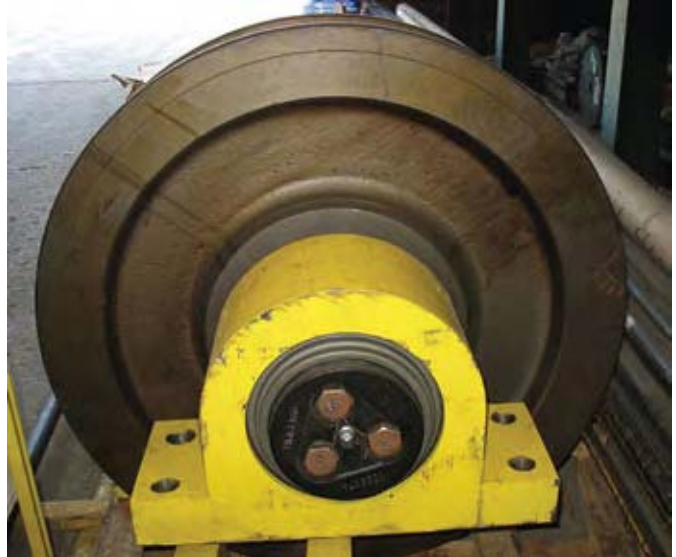
Fig. 12 AP bearings used in pillow block application
