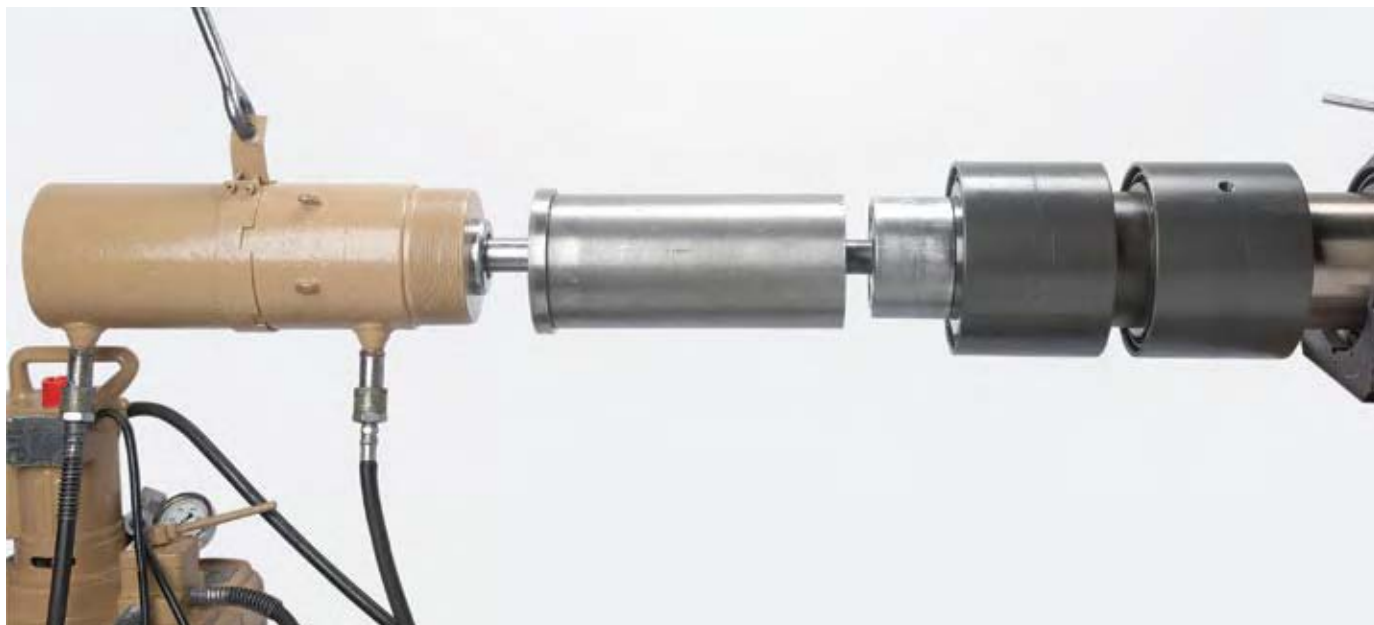
Fig. 28 Tooling used to push bearing onto shaft
